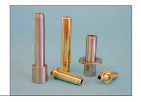
In one word: Performance. CHE valve guides use proprietary bronze alloys that exhibit excellent thermal conductivity and wear characteristics – but that's just the start. In an industry where the typical bronze valve guide is around .004 total indicator reading (T.I.R.), CHE uses its own tooling to produce valve guides that are .001 T.I.R. or less.
